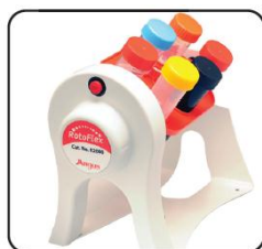
Change inserts to accommodate varying tube sizes
